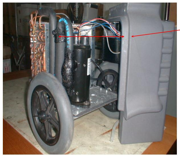
To remove back from chassis lift slightly, ease side away from refrigeration pipes lift clear ensuring wires do not snag or pull especially the sensor wire. Place down at an angle so that everything is accessible.
