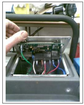
5 – Squeeze the plug on the other end of the defrost sensor wire and pull plug off control panel.
