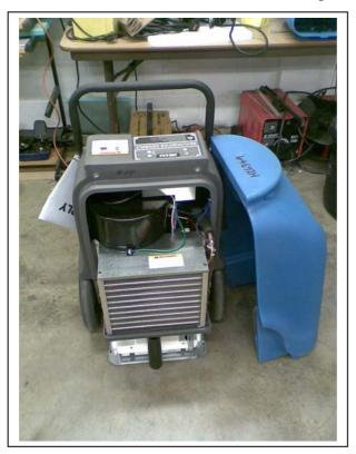
3 – Defrost sensor wire is thin blue wire on the right of the coil – remove the cable ties and pull the sensor out of the small pocket on the coil – see below
