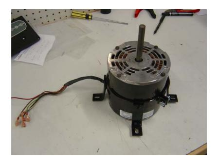
– Connect up wiring, refit fan to motor shaft making sure it sits 5 – 10 mm up off the motor, refit end guards and switch plate, and test – NOTE – on testing the fan is likely to blow out dust on initial startup – so point away from people
