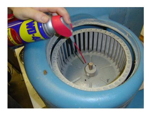
5 – Slide fan off motor spindle and out of plastic housing - see below
