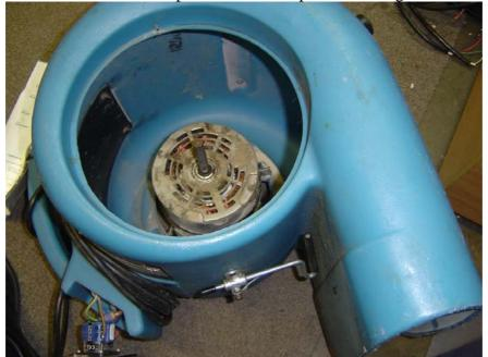
$6-Turn\ casing\ over\ and\ drill\ out\ 4\ rivets\ with\ 1/4"\ drill\ (\ 6.5mm\ )-see\ below$
