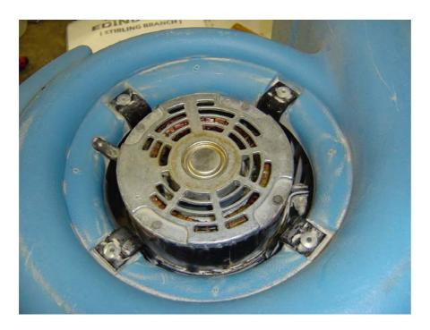
7 – Cut wires coming out of motor and old motor assembly will be able to be removed from plastic housing – see below for removed assembly
