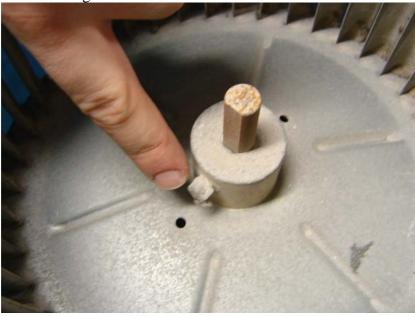
3- Using length of emery paper, clean up shaft of old motor to remove surface rust – see below
